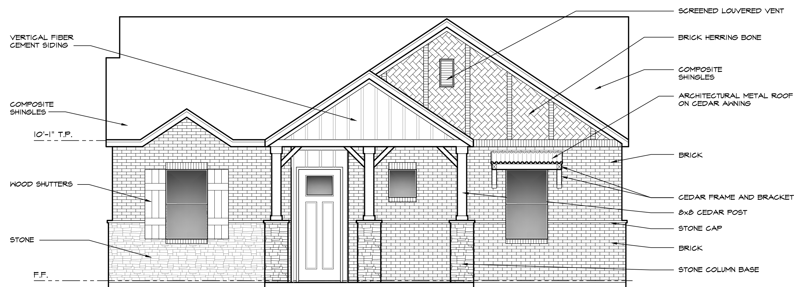
01 BUILDING TYPE "2" FRONT ELEVATION
