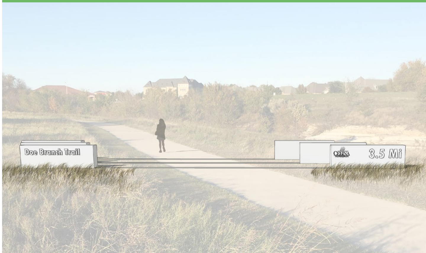
Figure 5.12, Potential Trail Mile Markers. Distinct trail markers should be provided along the trail network to aid in orienting users with their locations. Decorative paving may also be provided to enhance the design further.
